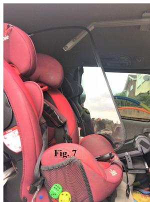
The only practical way of achieving this was to mount the screen over the right hand seat armrest, where the sister sat. Therefore, the first step was to profile the bottom of the screen to match the armrest. The top of the screen profile was later modified to remove sharp corners and the edging strip refitted. The complete installation is shown in the photo with the girls child seat in place.
