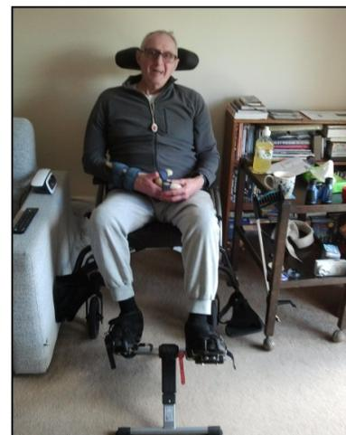
Footplates were formed and shaped to accept wide fitting bicycle toe-clips, the right one having to be longer to grip his affected foot more securely, these plates were also slotted at the sides to which long Velcro straps were fitted. The plastic pedals were drilled and the footplates bolted on.
