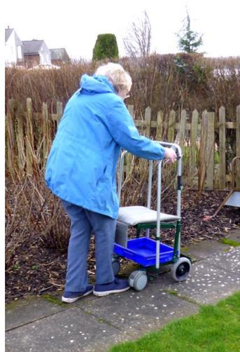
The ex-zimmer frame superstructure carried a hinged seat which acted as an automatic brake to the front wheels. These brakes were disabled by means of a cycle cable brake mounted on the upper tube, so that it was necessary to grip the brake to enable the frame to be moved. The castors also incorporate foot operated brakes. The frame allows the lady to access her raised beds and she can sit on it to carry out her gardening tasks.
