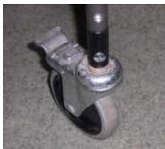
2" extension pieces were made to fit in the bore of each leg and around the castor base. They were secured by M6 bolts and nuts.
