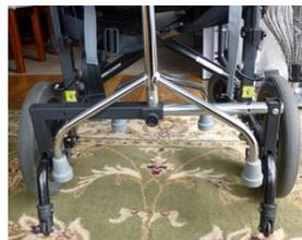
With the rod removed, the bridge to be telescopically reduced in size and the rod could then be refitted under the bridge to lock the assembly efficiently
