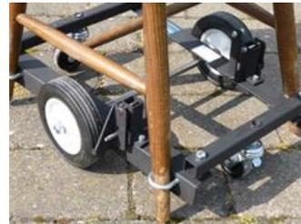
All four wheels on the chair were fitted with locking brakes. The wheel arrangement allowed the chair to be rotated around its vertical axis thus permitting its use in the very confined space available on board
