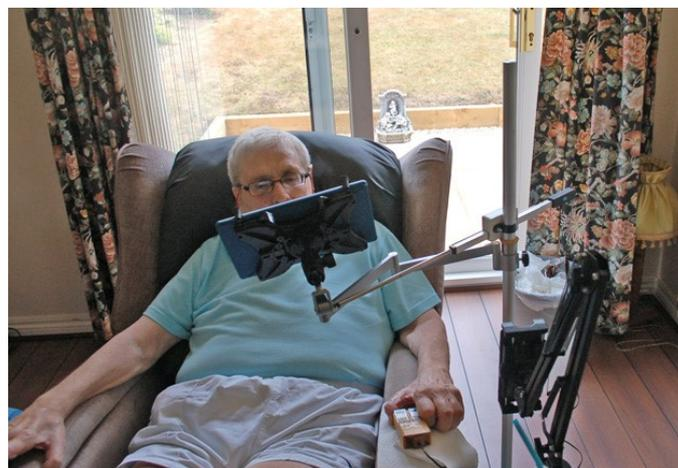
A 12 volt powered bespoke control panel and 2 channel relay system was made. It necessarily included very sensitive micro switches that he was capable of operating. A 12 volt DC power supply was also provided.
