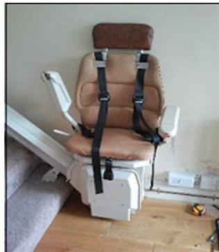
A headrest made from ply board was made that clipped over the seat top. Steel vertical support legs were bolted to the plyboard and through the seat back. The assembly was then covered with 10mm dense foam mat and soft padding on top, covered in brown vinyl.
