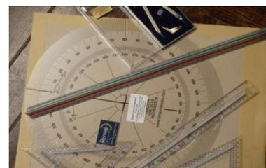
The solution provided by Brian Barry was to give the student a set of 'large' architect's instruments. The protractors are fitted with additional ribs which make it easier for the student to control their movement and the compass radius setting is controlled with a knurled screw and its 'centre' located by means of a separate marked perspex target plate.
