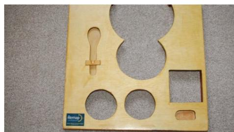
A Long Eaton blind lady needs a 'template stand' to hold the items she uses to prepare hot drinks in a known set arrangement. A paper template was provided by Sight Support staff. Malcolm Logan cut and fitted a matching plywood template.
