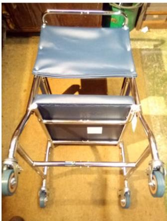
The casters were replaced with smaller ones with stainless adapters to accept the replacement castors, threaded fixing M12, thus lowering the chair by 50mm.
