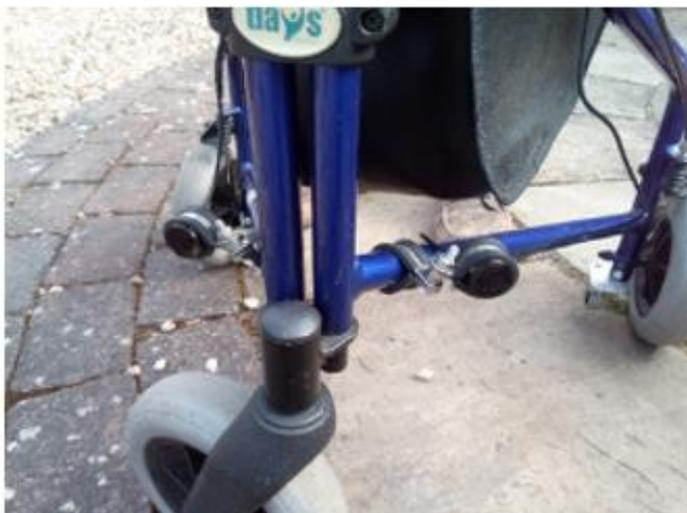
A solution based on car parking sensors was investigated. A pair of sensors were fitted to the rollator along with vibration motors in the hand grips. A processor unit was programmed to read the sensors and when an obstacle is sensed, one or both hand grips will vibrate.
